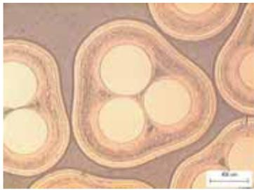
Fig. 3. Optical micrograph for the cross-sections of the agglomerated particles.
