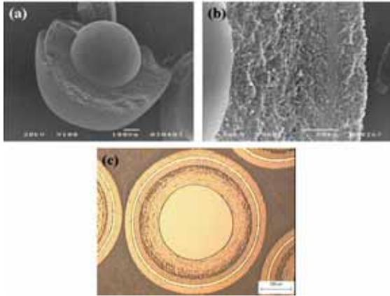
Fig. 2. Fractured ((a) and (b)) and polished (c) cross-sectional micrographs of the TRISO coated particles.
