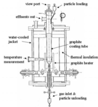
Fig. 1. Schematic diagram of the FBCVD coater.
