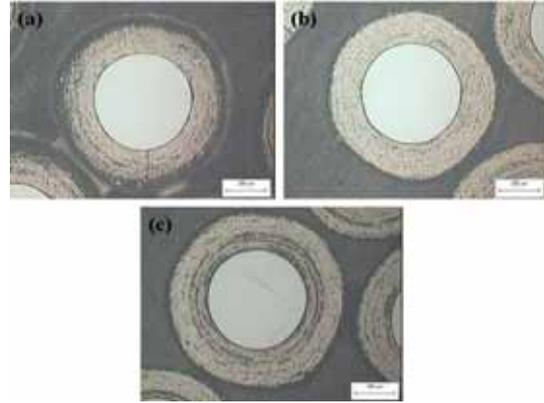
Fig. 4. Optical micrographs for the cross-sections of the buffer coated particles with the flow rates of 1700 (a), 2000 (b), and 2500 sccm (c).
