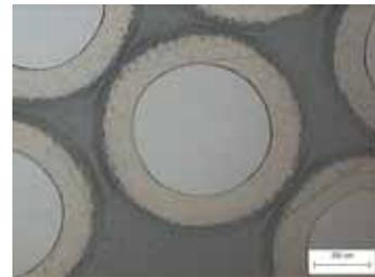
Fig. 5. Optical micrograph for the cross-section of the buffer coated particles with the C<sub>2</sub>H<sub>2</sub> concentration of 50%.
