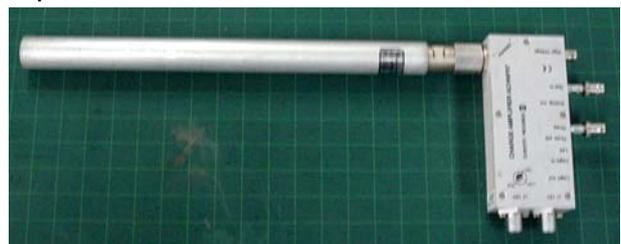
Figure 2. Layout of the He-3 proportional counter and preamplifier for signal processing.
