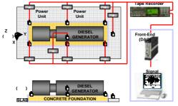
Fig. 3. Schematic Diagram of Measurement System
