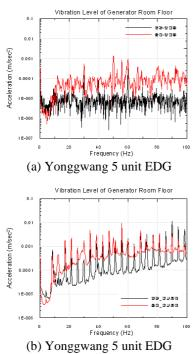
Figure 4. Frequency Response of EDG at the Floor<sup>[1]</sup>
