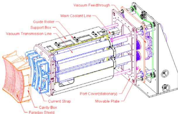
Figure 1. Detail 3-D drawing of the ICRF antenna.
