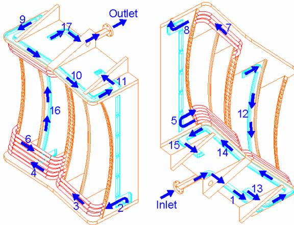
Figure 3. Cooling path diagram for the Faraday shield and the cavity walls.
