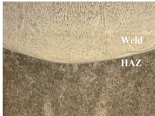
- Figure 4. Microstructure after welding with developed equipment(peak current : 140A, base current : 70A, welding speed : 180mm/min and wire feeding rate : 1,100mm/min)
