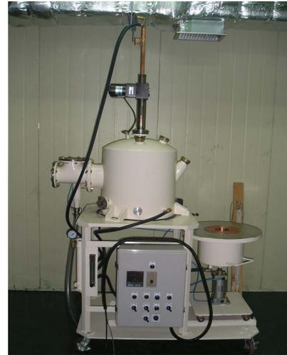
Figure 1. Electric arc melting apparatus.
