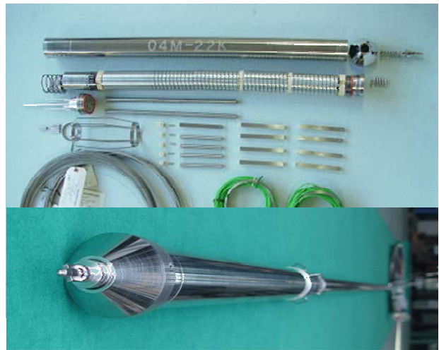
Figure 3. Parts and assembled one of a fluence control capsule.
