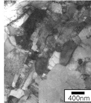
Figure 1. Bright field TEM image of as-extruded Zr-1Nb alloy.
