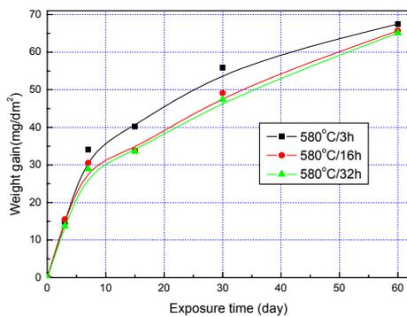
Figure 2. Influence of annealing duration on the corrosion behavior of Zr-1Nb alloy at 400°C in steam.
