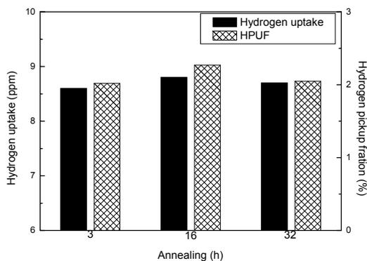
Figure 3. Hydrogen uptake and hydrogen pickup fraction of Zr-1Nb alloys after corrosion for 60 days.
