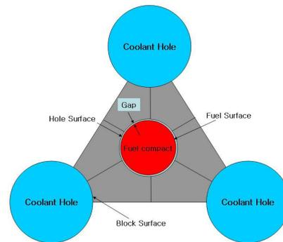
Figure 2. Unit coolant channel model in the PMR assembly.
