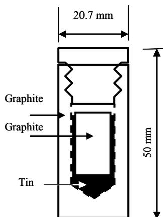
Figure 4. Shape and dimensions of the sample used for the compatibility study.
