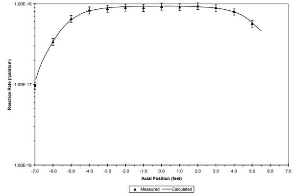
Figure 1. comparisons of  $^{54}\text{Fe}(n,p)^{54}\text{Mn}$  reaction for bead chain installed at azimuthal angle 0 degree for YGN-1
