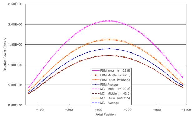
Figure 6. Comparison of axial power distributions
