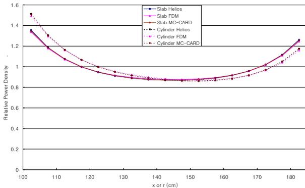
Figure 3. Power distributions of the 1-D problems
