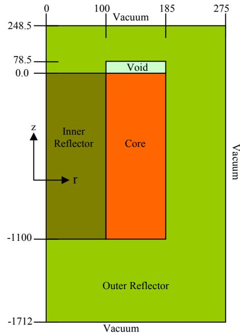
Figure 1. Geometry and dimensions of the problem
