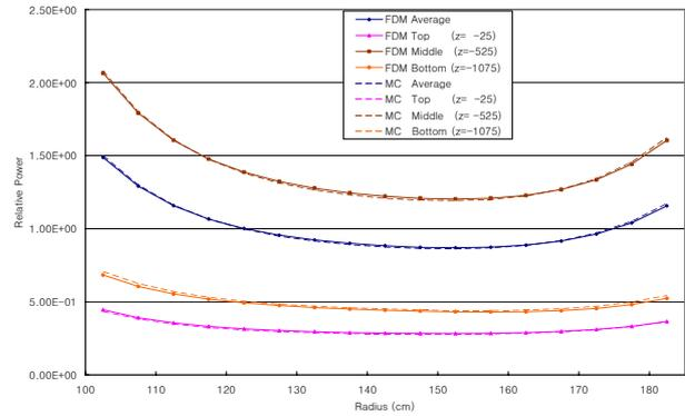
Figure 5. Comparison of radial power distributions
