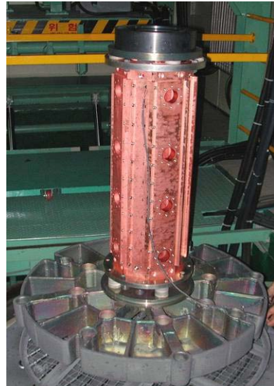
Figure 2. RFQ section prepared for brazing
