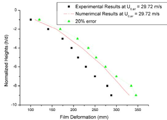
Figure 4. Calculated film deformation at  $u_{0,air} = 29.72$  m/s.
