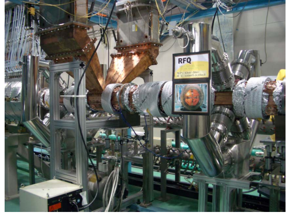
Figure 4. Installed RFQ upgrade
