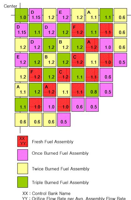
Figure 2. Loading Pattern of a Equilibrium Core with Control Banks Position and Orifice Flow Rate
