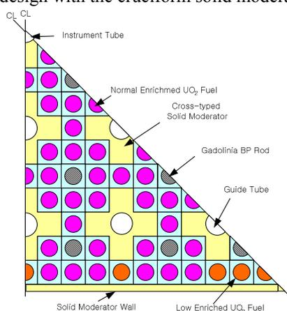
Figure 1. A Conceptual Assembly Design
