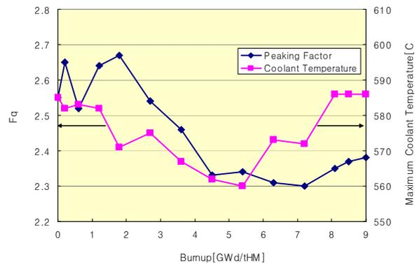
Figure 3. Fq and Max. Coolant Temperature vs. Burnup
