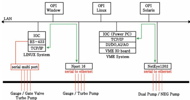
Figure 2. PEFP Vacuum Control System Architecture.
