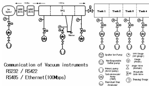
Figure 1. Lay out of vacuum system at front end.
