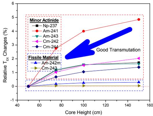
Fig. 2 Change in relative T<sub>EX</sub> to core height
