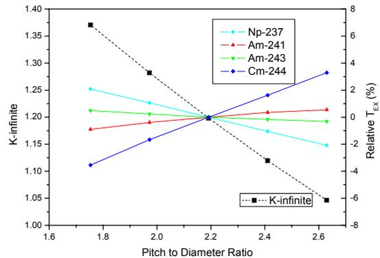
Fig. 1. Change of K-inf and relative  $T_{EX}$  to P/D Ratio
