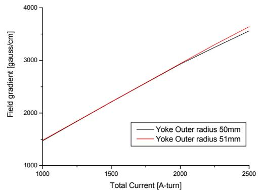
Figure 2. Field gradient of the EQM dependent on current
