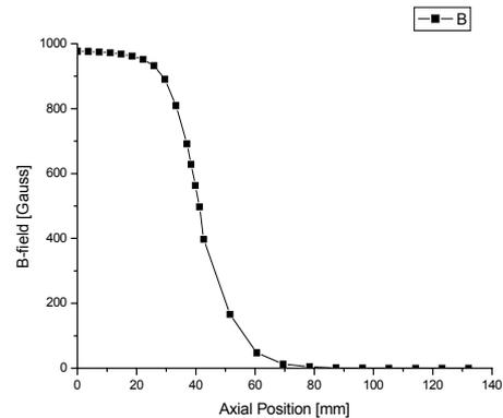
Figure 3. Axial distribution of the quadrupole field of the EQM
