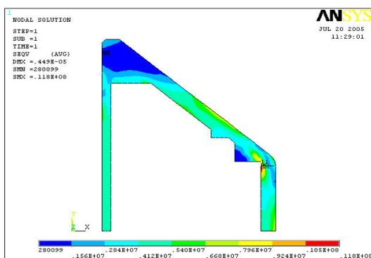
Figure 4. Result of the structural analysis : the Equivalent stress.
