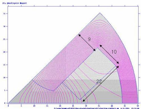
Figure 1. 2-D modeling of the magnetic calculation for the EQM
