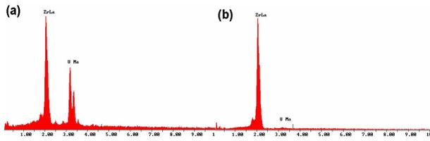
Figure 2. SEM micrograph and EDS analysis results for U-55wt%Zr sintered sample. (a)  $\delta$ -UZr<sub>2</sub> matrix, (b)  $\alpha$ -Zr phase.
