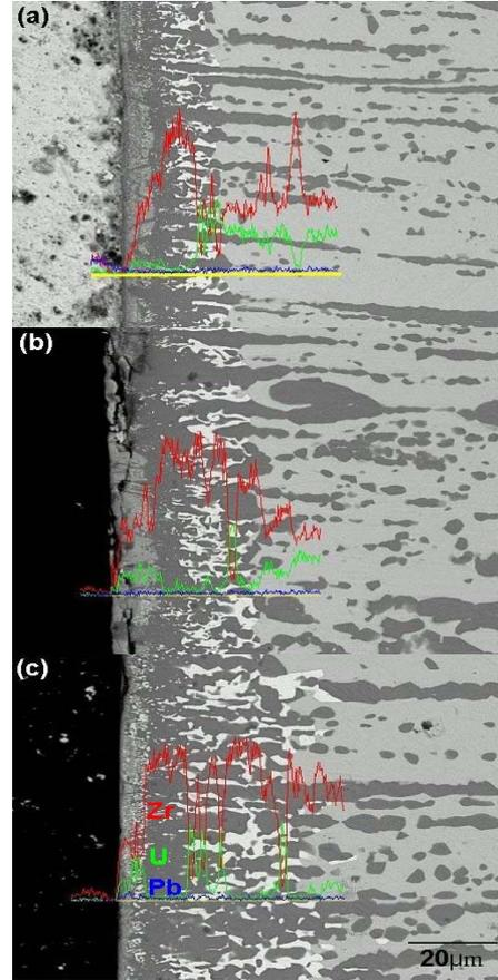
Figure 4. Line profiles of the interface of the U-55Zr fuel with a Pb bonding according to the annealing time at 650°C. (a) 100hr, (b) 200hr, (c) 1000hr.
