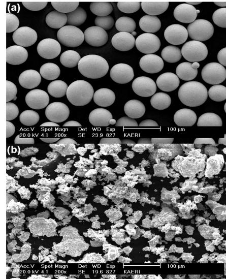
Figure 1. Photographs of the atomized U powder(a) and Zr powder(b).
