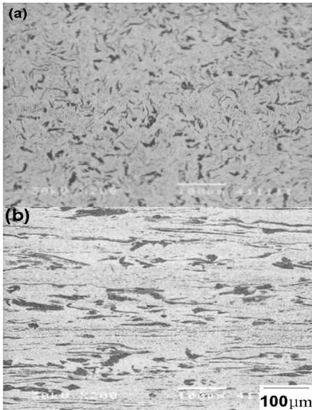
Figure 3. SEM micrographs of the extruded rod. (a) transverse direction, (b) longitudinal direction.
