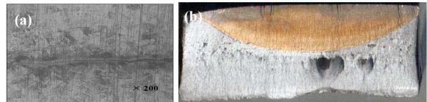
Figure 2. The crack by mechanical method (a) fatigue crack (b) fracture surface
