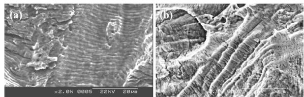
Figure 4. SEM fractographic of mechanical and thermal stratification method (a) Mechanical fatigue crack (b) Thermal fatigue crack
