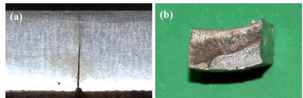
Figure 3. The crack by thermal stratification method (a) Thermal fatigue crack (b) fracture surface
