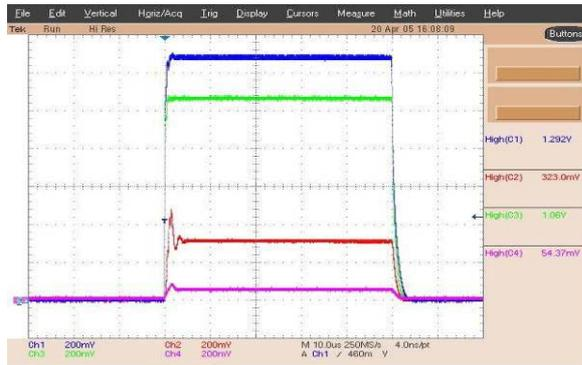
Figure 4: The measured RF signal in HPRF test for the DTL klystron
