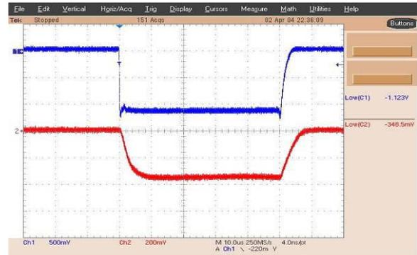
Figure 2: The measured RF signal in the HPRF test for the 3MeV RFQ
