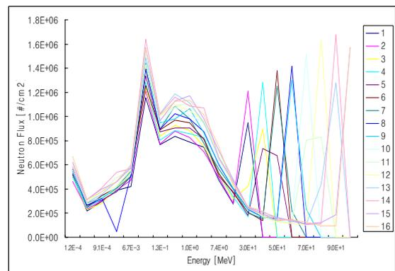
Figure 2. The Neutron Spectra in the 20~100 MeV DTL tanks 16 units
