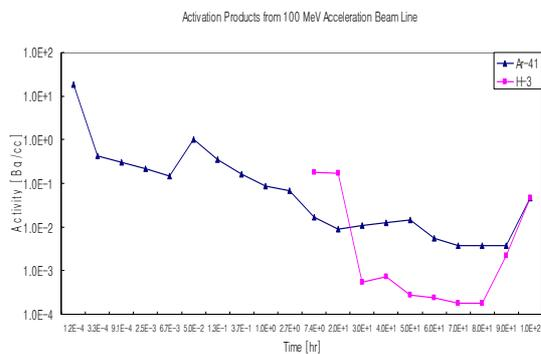
Figure 3. The Production Rate of the Activation Products in Air
