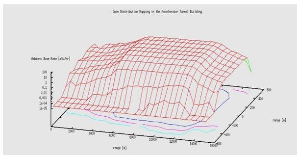
Figure 4. The Ambient Dose Distribution Map in the Accelerator Tunnel Building for Prompt Radiation Field
