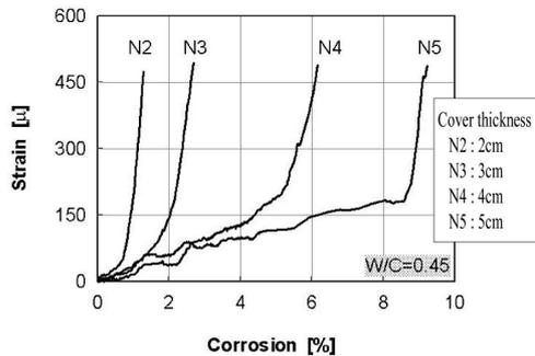
Figure 3. Surface strain-corrosion relationship for cover thickness [2]
