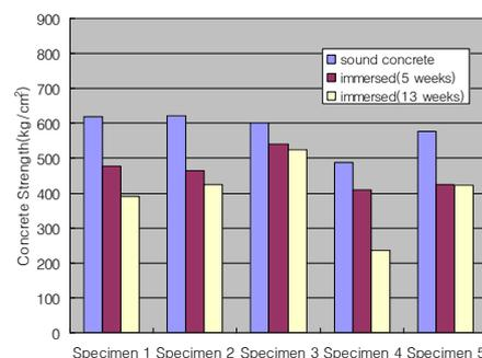
Figure 2. Graph for concrete strength verses specimen type for different immersing times
