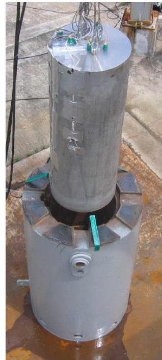
Figure 1. Free drop test of a canister onto the concrete pad of the overpack.
