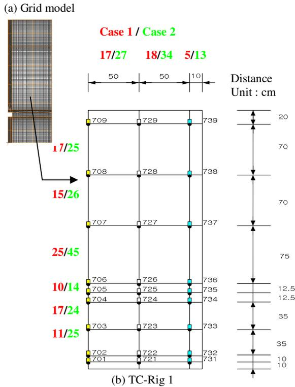
Fig. 1. Grid model and the mesh distribution
