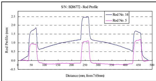
Fig1 Outer Rod Profile of B206772 PI Bundle
