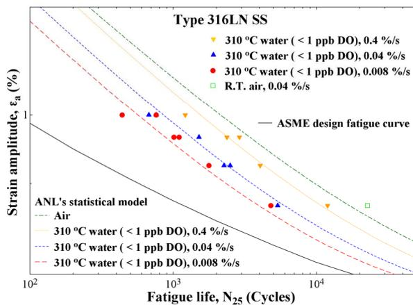
Figure 3.  $\epsilon$ -N curves of type 316LN SS in 310 °C low oxygen-containing water.
