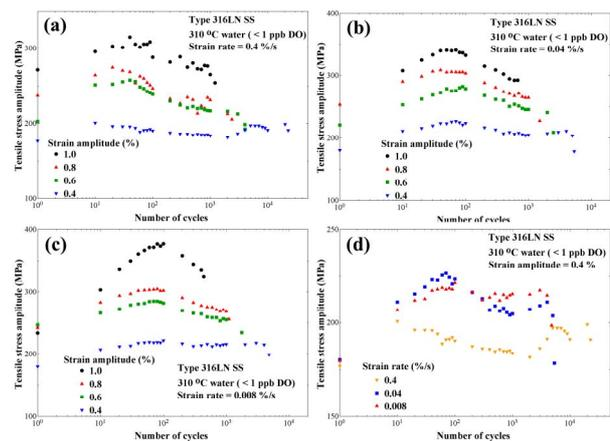
Figure 1. Cyclic stress response of type 316LN SS in 310 °C low oxygen-containing water at strain rates of (a) 0.4 (b) 0.04 (c) 0.008 %/s, and (d) three strain rates at 0.4 %.
