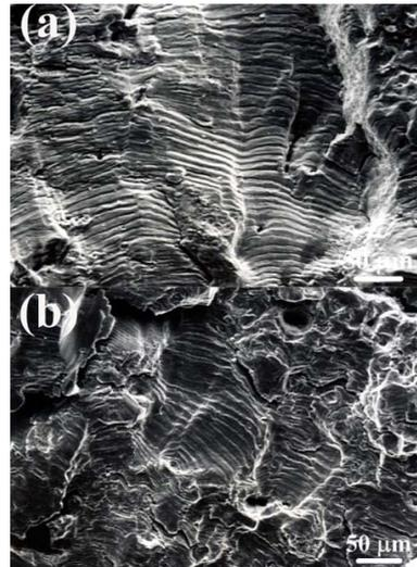
Figure 4. Fatigue surface morphology of type 316LN SS in 310 °C low oxygen-containing water at strain rate of (a) 0.04 and (b) 0.008 %/s.
