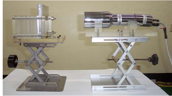
Fig. 1. Experimental setup for dual energy gamma-ray system.
