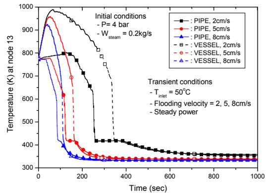
Figure 5. Comparison of wall temperature between the PIPE and the VESSEL modeling
