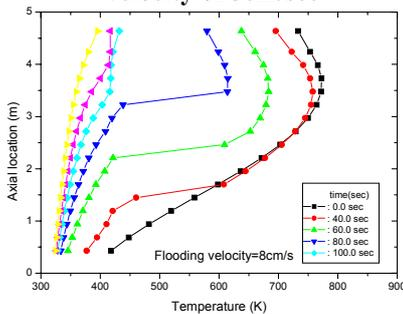
Figure 4 Wall temperature profile for flooding velocity of 8cm/sec
