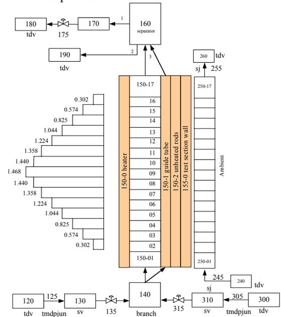
**Figure 1. PIPE module nodalization for the 6x6 reflood test section**
