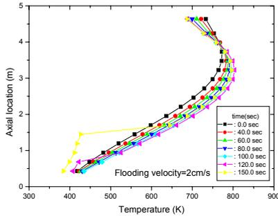
Figure 2. Wall temperature profile for flooding velocity 2cm/sec
