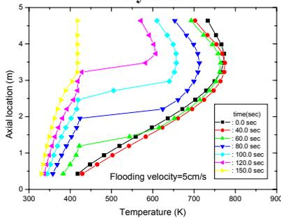
Figure 3 Wall temperature profile for flooding velocity of 5cm/sec
