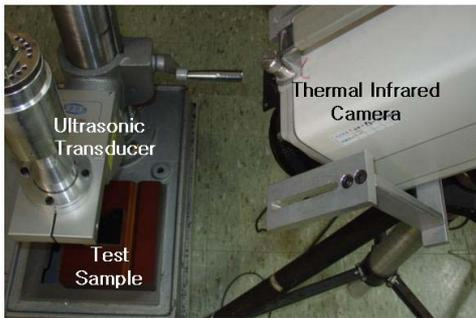
Fig 2. Experimental setup of lock-in thermography with ultrasonic excitation.
