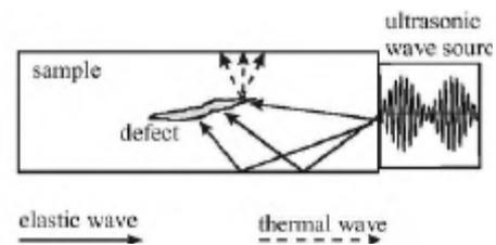
Fig 1. ULT principle: Modulated ultrasound excitation generates thermal waves in the defect itself, those are sensed at the surface (courtesy of G. Busse).
