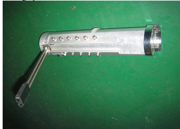
Figure 2. KALANS ® -III Nozzle Head Assembly
