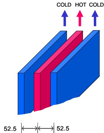
Figure 1. The shape of the triple jet nozzles
