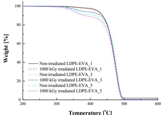
Figure 1. TG thermograms of  $\gamma$ -ray irradiated LDPE/EVA blends.
