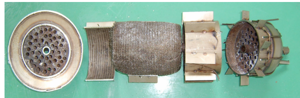
Figure 4. Cold trap after sodium removal by the nitrogen-superheated steam
