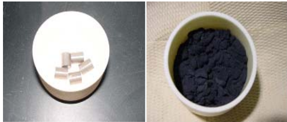
Figure 3. \text{UO}_2 pellets and \text{U}_3\text{O}_8 powders of a vol-oxidation experiment
