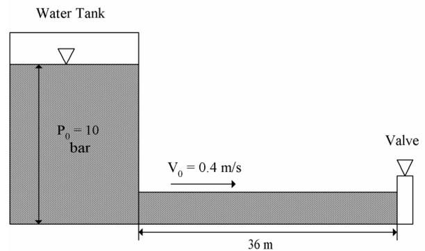
Figure 1. The water hammer experiment
