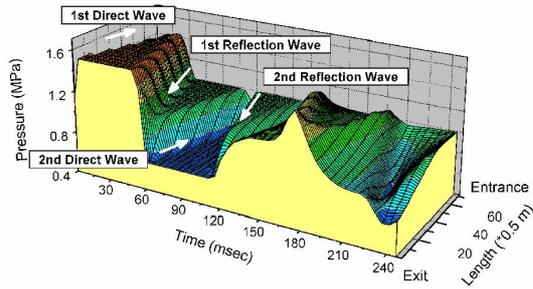
Figure 3. Pressure wave propagation along the pipe with time
