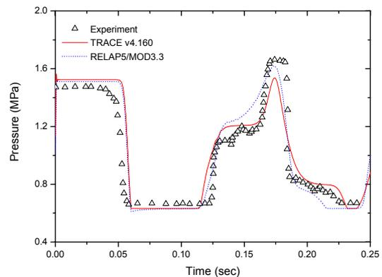
Figure 2. Comparison of pressures at the valve of the water hammer experiment
