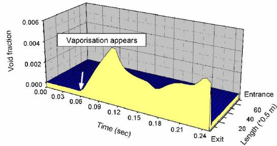
Figure 4. Void fraction distribution along the pipe with time
