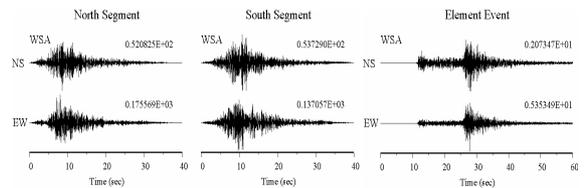
Fig. 4 Synthetic Ground Motions (left, center) and the Observed Records (right) at WSA.
