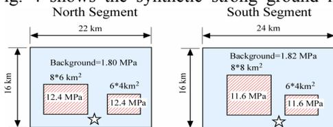
Fig. 2 Assumed Source Models for the Ulsan Fault
