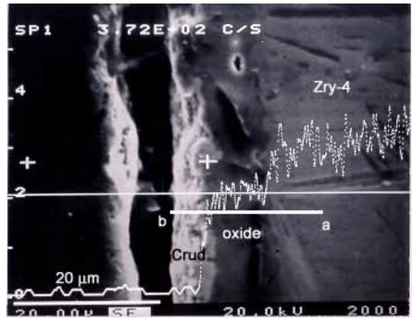
Figure 2. Inner surface of cladding hull (SEM) and Zr concentration profile.
