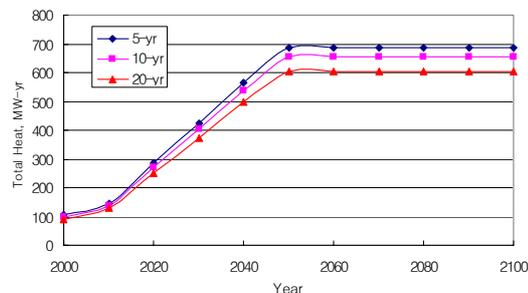
Fig. 2 Comparison of total heat load for different cooling times of the CANDU SF
