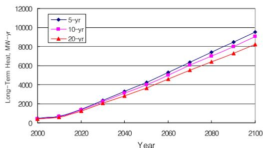
Fig. 1 Comparison of total heat load for different cooling times of the PWR SF
