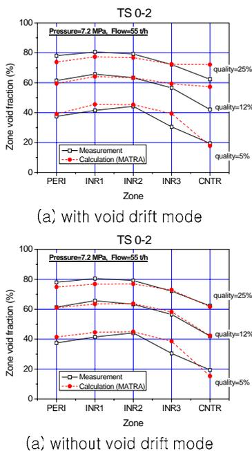
Figure 3. Effect of the void drift model for a test bundle with four unheated rods
