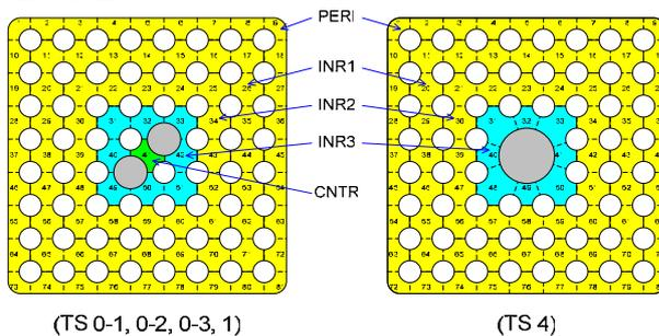
Figure 1. Cross-sectional view of the 8x8 test bundles.
