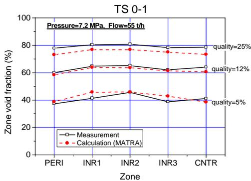
Figure 2. Radial void distribution in TS 0-1
