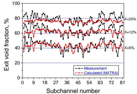
Figure 4. Subchannel void distribution in TS 4.
