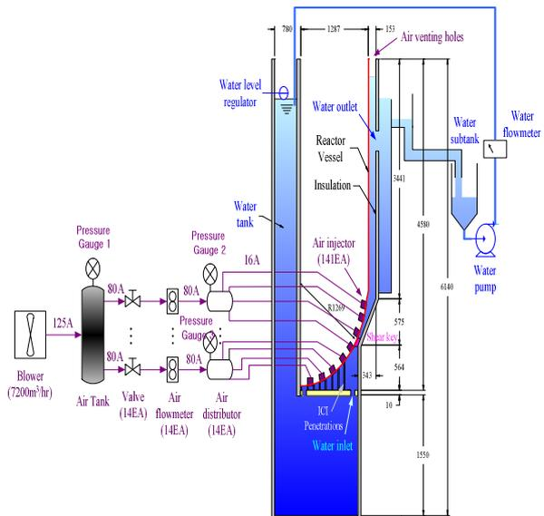
Figure 1. Schematic diagram of the HERMES-HALF experimental facility.
