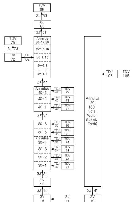
Figure 2. RELAP5 input model for the HERMES-HALF experiment.
