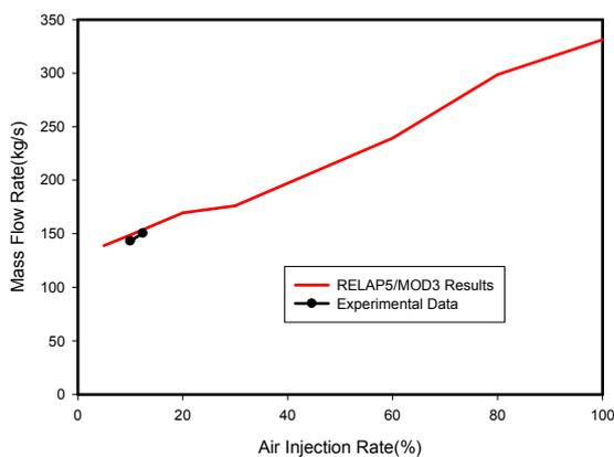
Figure 4. RELAP5 results on the water circulation mass flow rate as a function of air injection rate at large water inlet area.
