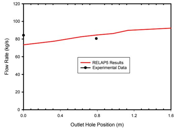
Figure 5. RELAP5 results on the water circulation mass flow rate as a function of water outlet position.
