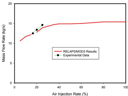
Figure 3. RELAP5 results on the water circulation mass flow rate as a function of air injection rate at small water inlet area.
