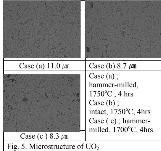
Fig. 5. Microstructure of UO<sub>2</sub>
