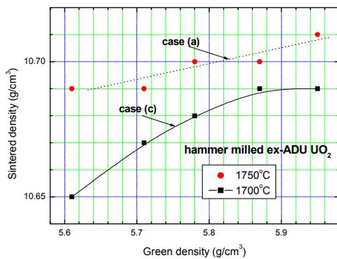
Fig. 4. Green density vs. sintered density with 2 different sintering temperatures.
