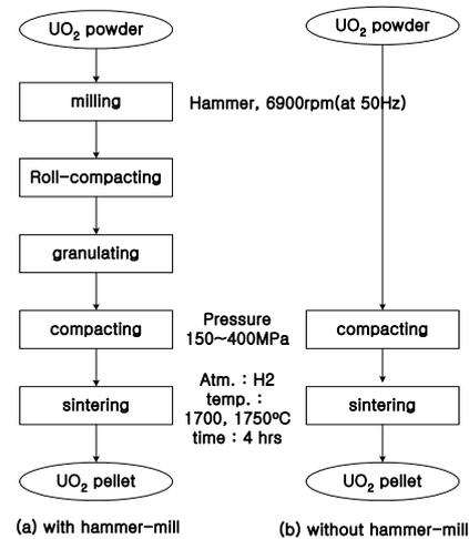
Fig. 2.  $\text{UO}_2$  pellet fabrication route
