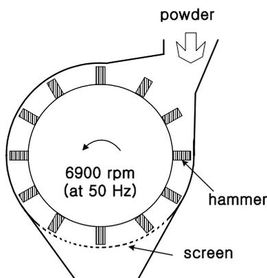
Fig. 1. A schematic diagram of a hammer mill
