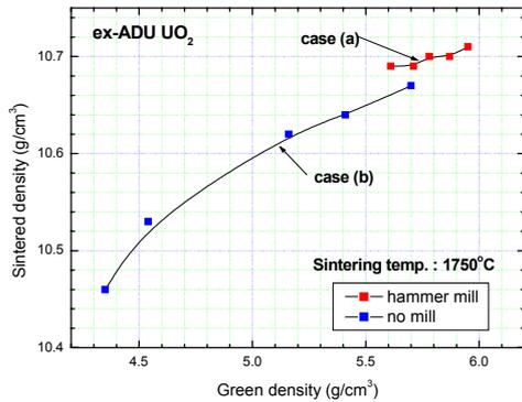
Fig. 3. Green density vs. Sintered density as a function of milling effect.
