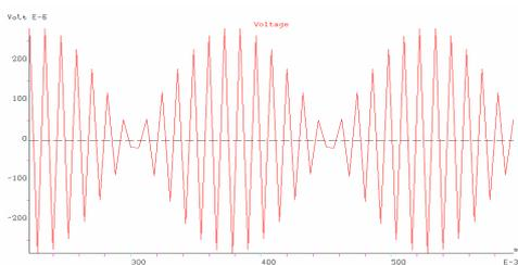
Figure 7. Induced Voltage Result of Sensor with Radially Magnetized Permanent Magnet.
