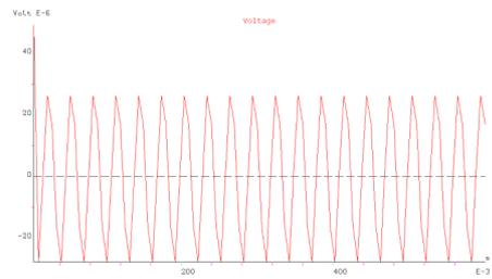
Figure 5. Induced Voltage Result of C-shaped Sensor.
