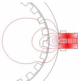
Figure 5. Equi-flux Lines Result of C-shaped Sensor.
