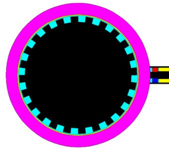
Figure 1. Sensor with Radially Magnetized Permanent Magnet.
