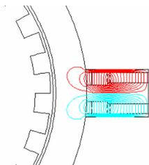
Figure 4. Equi-flux Lines Result of Sensor with Radially Magnetized Permanent Magnet.
