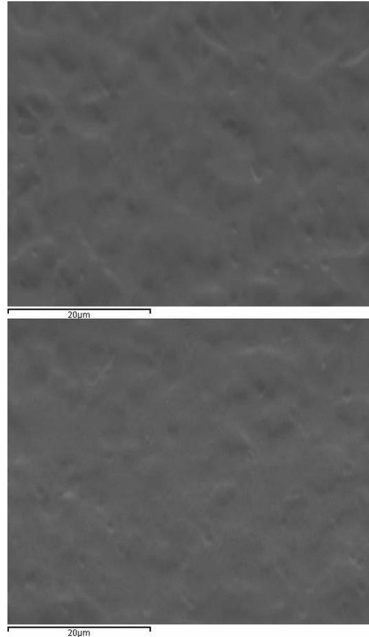
Figure 1. Cross sectional view of 2<sup>nd</sup> pilgered zirconium alloy tube observed by scanning electron microscopy : (top) center (bottom) inner area
