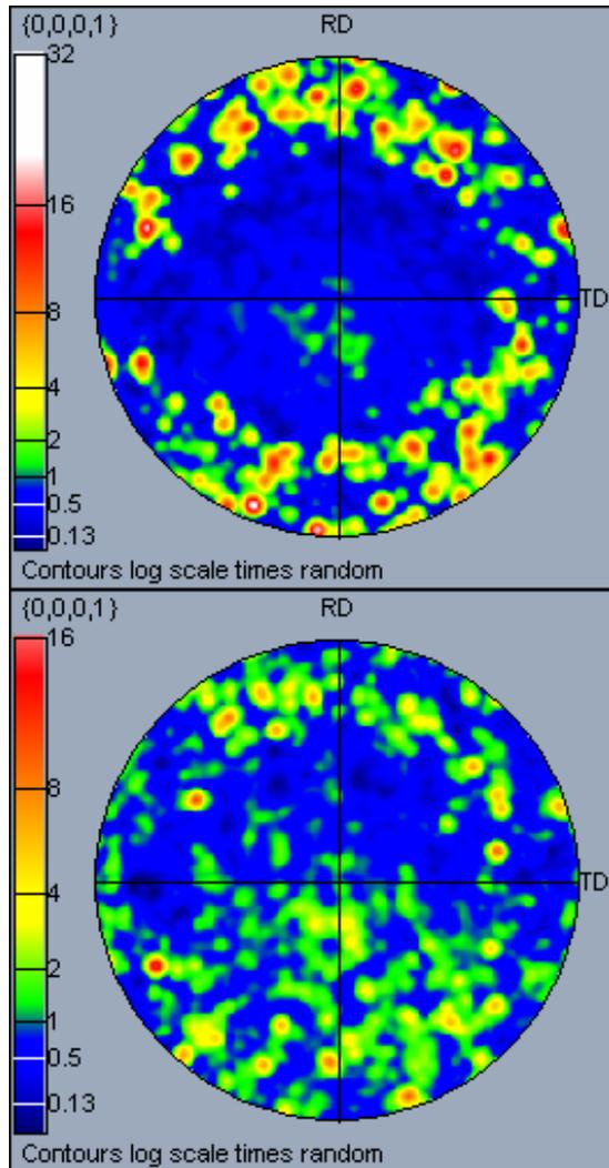
Figure 2. (0002) pole figures of grains in 2<sup>nd</sup> pilgered zirconium alloy tube : (top) center (bottom) inner area
