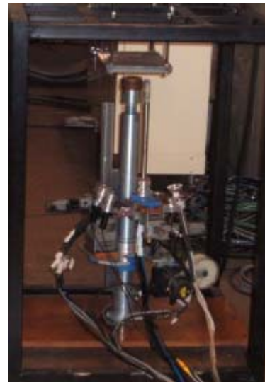
Fig.2. The Welding Equipment for CRD Nozzle Welds.
