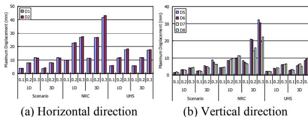
Figure 6. Comparisons of displacement responses for the isolated EDG.
