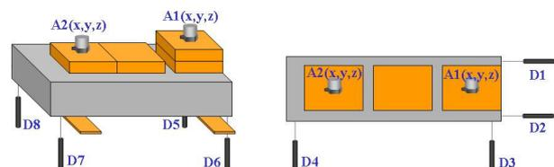
Figure 4. Arrangement of accelerometers and LVDTs.
