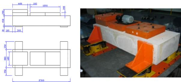
Figure 1. EDG model for shaking table tests.
