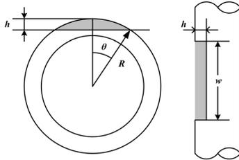
Figure 2. Wear topology (flat wear)
