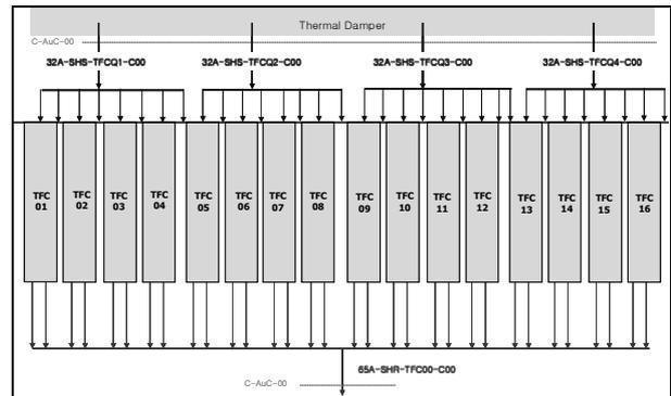
Figure 1. TF coil flow diagram
