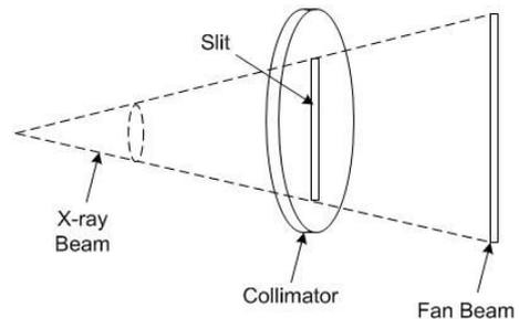
Figure 4. MCNP Modeling of Fan X-ray Beam
