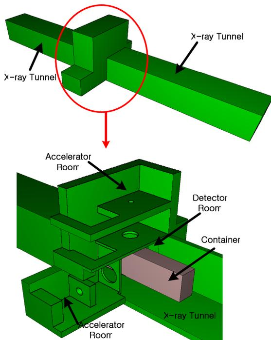
Figure 3. MCNP Modeling of Inspection System
