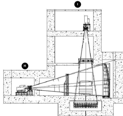
Figure 2. Vertical View of the Container Inspection Facility
