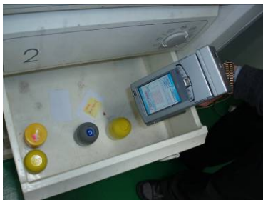
Fig.2. Reading RF tag in refrigerator (at - 20°C)
